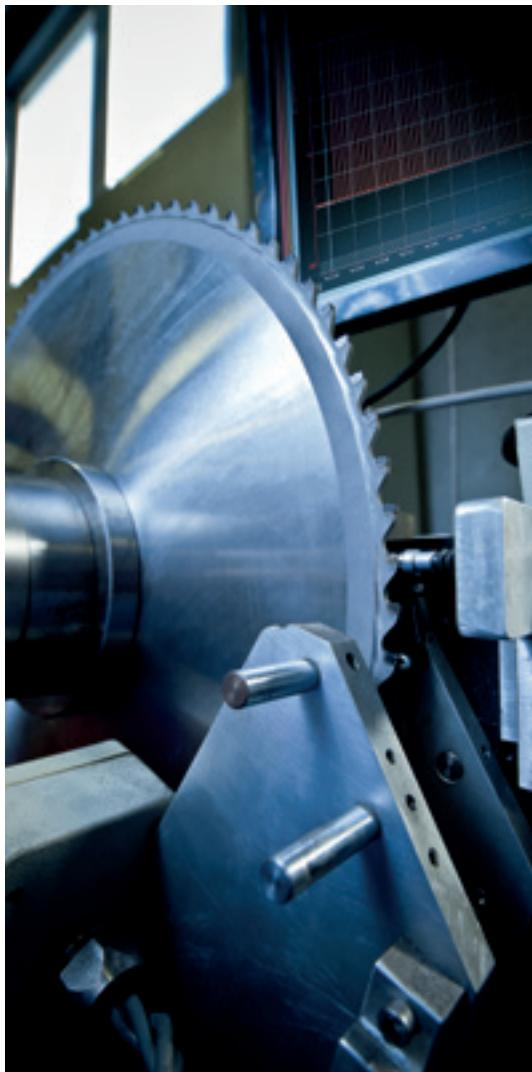
All Julia's products are tested before being delivered to the customer. The dimensional tolerances for the HM and Cermet saws are checked 100% of the time. The final test includes the teeth concentricity, the side clearance, the geometry and the central bore dimension.
